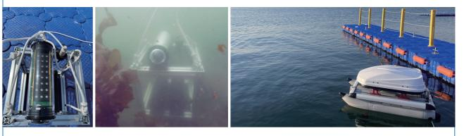
A platform designed to collect and store underwater video or sensor data on a regular basis for a certain period of time. Data can be collected separately using an unmanned vessel, not collecting the platform itself.
